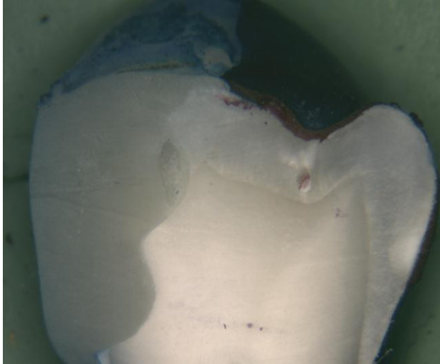
Figure 7: Group 6, CHX gel G-bond and gradia direct posterior composite restoration group gingival and occlusal microleakage value =0 (x15)
